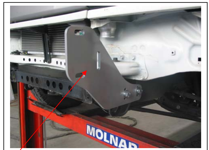
8mm steel mounting plate Figure 2 – Passenger side shown
